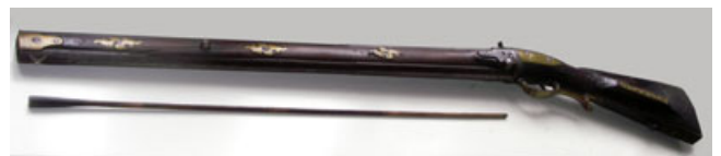
FIG. 1—Muzzle-loader and ramrod (around 1800). Preparing the discharge, the ramrod is used to compress the black powder and to push the bullet down to the bottom of the barrel. While not in use, the ramrod is kept in a sheath below the barrel. Depending on the model of the weaponry, the ramrod itself is made of steel or wood.
